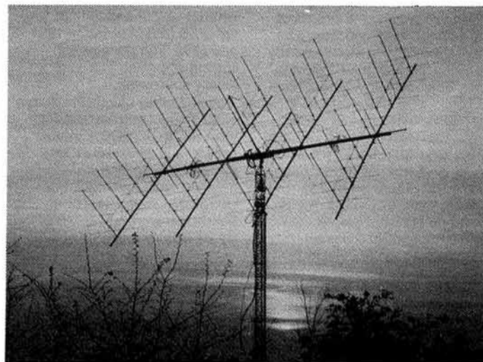
The 224-element colinear array used by G8MBI for 144MHz moonbounce.
